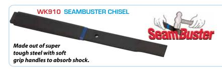
These Heavy-Duty chisels allow you to easily separate pre-drilled welded or bonded panels. Sharpened on 2 edges – sharp end allows for penetration between panels and the side edge allows for side impact to separate panels without damage.
