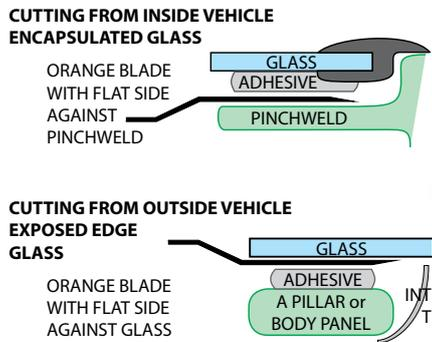
**NOTE!** Orange and Blue Reverse 'R' Blades have the cutting tip bent opposite to the Yellow blades
