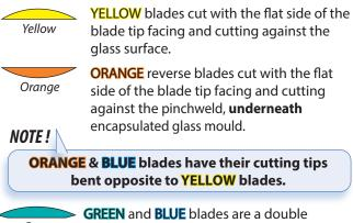
*Green* bevelled safety-edge version of **YELLOW** and **ORANGE** blades respectively. See the V blades section on Page 28 for further details.
