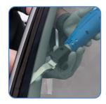
TIP Non-Serrated offset blades can also remove body side mouldings, emblems, decals and nameplates.
